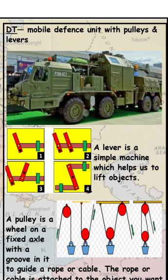
to guide a rope or cable. The rope or cable is attached to the object you want to lift and looped over the pulley so that the end of the rope is hanging down on the other side. The pulley changes the direction of the force needed to lift the object or the amount of force that is needed to lift an object.
